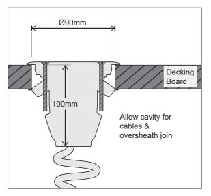
Ø90mm cutout is required for installation into decking. Canister is not required when installing into decking.
