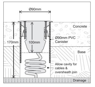
Fitting is supplied with a Ø90mm PVC Installation Canister. Canister can be placed in slab prior to concrete pour to ensure good drainage to sub-soil.
