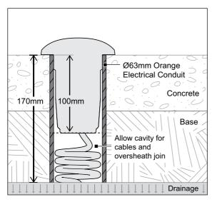
Fitting is compatible with many Ø63mm Orange Electrical Conduits and may offer a preferred installation option. Mounting Collar is not required in this instance.
