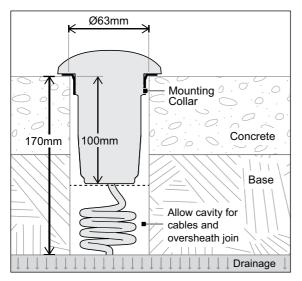
Fitting is supplied with a Mounting Collar to suit a Ø63mm cored hole.
