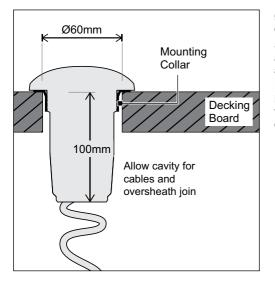
Ø60mm cutout is required for installation into decking. Use Mounting Collar supplied.
