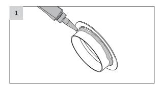
Apply appropriate adhesive on the underside corner/lip of the collar.
