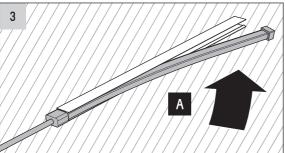
To assemble Strip Light into Channel Mount:
