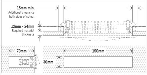
Cut-out for 210mm Step Light is 190mm (W) x 30mm (H) x 70mm (minimum depth) to ensure sufficient space for connector and cable behind light fitting when installed.
