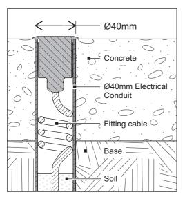
Fitting will mount into grey 40mm PVC electrical conduit. Canisters can be placed in slab prior to concrete pour to ensure good drainage to soil.
