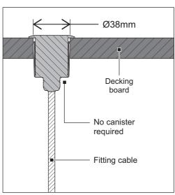
Ø38mm cutout is required for installation into decking. No canister is required.
