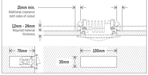
Cut-out for 120mm Step Light is 100mm (W) x 30mm (H) x 70mm (minimum depth) to ensure sufficient space for connector and cable behind light fitting when installed.
