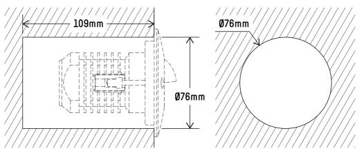
Cut out for Step Light is Ø76mm x 109mm (minimum depth) to ensure sufficient space for connection and cable behind light fitting when installed. Hole size is a standard core drill bit or hole saw size. If install canister is required fitting will mount into 75mm PVC plumbing pipe.
