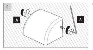
10 A B C Feed cable Attach fitting assembly to Base Plate by tightening two Grub Screws using Hex Tool (supplied) (A).
