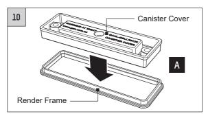
Assemble Canister Cover into central opening in Render Frame (A).
