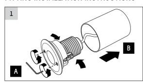
To release fitting from canister:
