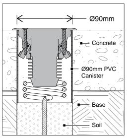
Fitting is supplied with a Ø90mm PVC installation canister. Canisters can be placed in slab prior to concrete pour to ensure good drainage to soil.
