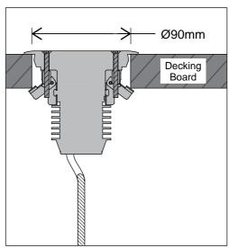
Ø90mm cutout is required for installation into decking. Discard installation canister when installing into decking.
