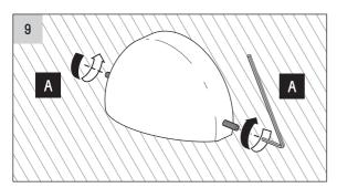
Attach fitting assembly to Base Plate by tightening two Grub Screws using Hex Tool (supplied) (A).
