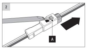
Separate IP67 connector by pushing on locking tab (A) with small flat blade screwdriver.
