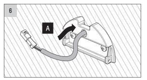
Insert cable with connector through Base Plate and wall via central hole in Base Plate (A).
