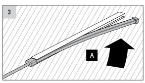
To assemble Strip Light into Mount Channel:
